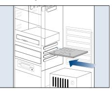
4. Secure the controller card bracket to the system case.
